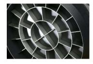
Anodized coated aluminium dividing disc and stainless steel knife require minimal flour for dividing and are hygienic in use.
